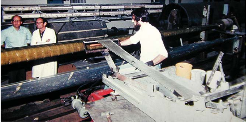
Figure 8 Tape winding of a spar for the Nibe wind turbines. The thickness of the spar was varied along the length, by varying the length of travel of the tape placement apparatus along the length of the spar. A wedge was manually inserted and withdrawn underneath the tape, at the shear web position of the spar, for each revolution of the mandrel, in order to control and maintain straight fibers with the desired orientation in the upper and lower part of the spar.
